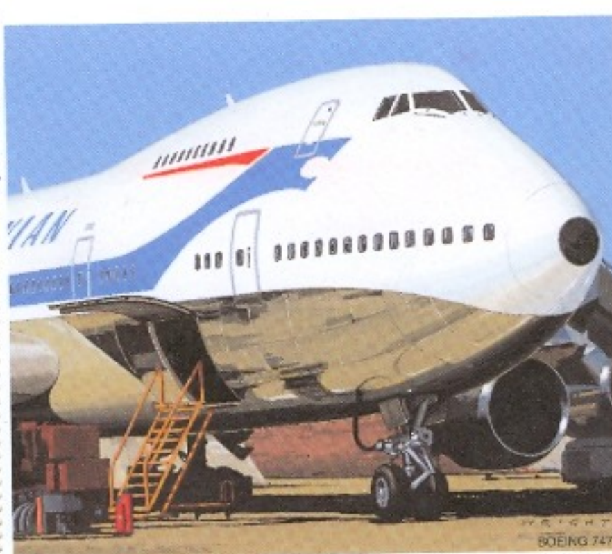
BOEING 747 THE FIRST "JUMBO JET" OF THE AIR. THE BOEING 747 CAN CARRY UP TO 400 PASSENGERS. IT IS POWERED BY FOUR TURBOJET ENGINES AND ITS TOTAL LENGTH IS 235 FEET. THE BOEING 747 IS FLOWN BY MOST OF THE WORLD'S MAJOR AIRLINES.
